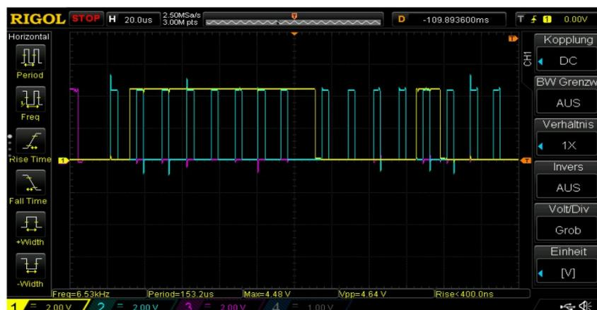
Pin Clock (CLK) has the color cyan, the data pin the color yellow. Pin Chip Enable (CE) has the color magenta. You can see the transmission of 2 bytes after CE goes to LOW.
